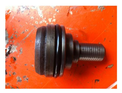
Changing the seals and shims is a 20 min job, getting the PR off and putting it back on the car can take a lot longer than that depending on which model it is! But this is an easy DIY job really and a good way to get the system pressure right. My XM is now cutting out at 172 bar and cutting in at 147 bar, which seems to me to have sharpened the brakes a little and smoothed the ride a shade too!
