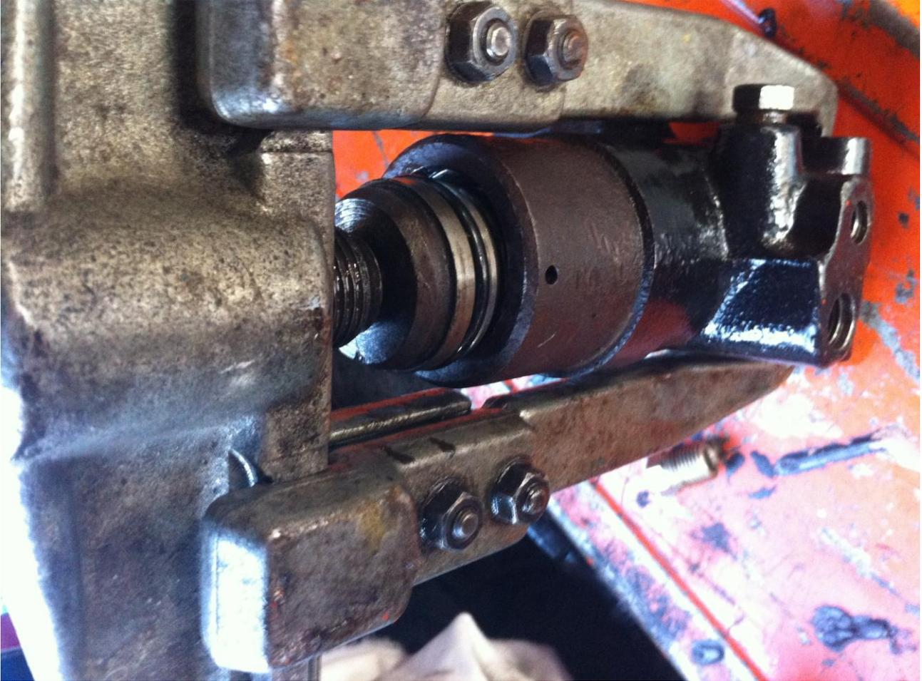
On the top of the spring is a thick end cap with a peripheral seal. The O ring is smaller and fatter than the other one - it measures 29 x 34.4 x 2.7mm. Between the end cap and the spring are washer shims - they measure 32mm OD and 24.5mm ID. Again the seal is easy to replace and the shims can be adjusted as before. Reassembly is the reverse process, just need to be careful to ensure the assembly enters the hole centrally as it's depressed, pop the circlip back in and release.
